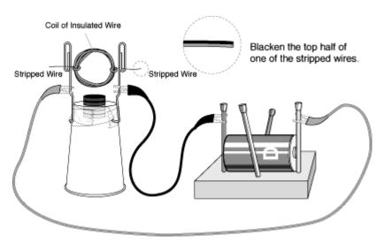
If you are using insulated wire, strip the insulation off the ends of the wire projecting from the coil. If you are using enameled wire, use the sandpaper to remove the enamel. Color one side of one of the projecting ends black with the marking pen. (Note: It is very important that the orientation of the painted side corresponds to the orientation shown in the drawing. If the coil is held in a vertical plane, paint the top half of one of the wires black.)
